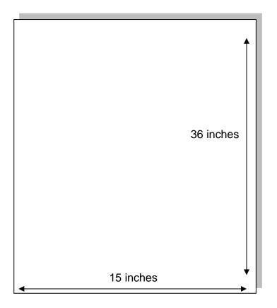
When measuring windows, measure ONLY the area that a person would actually use as an exit. The square footage of the exit/egress MUST be a minimum of 3.77 sq.ft. If 1 dimension is the minimum height OR width of 15", the other dimension MUST be a minimum of 36".
